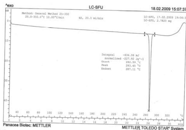
Fig. 6: DSC plot of 5-Fluorouracil
